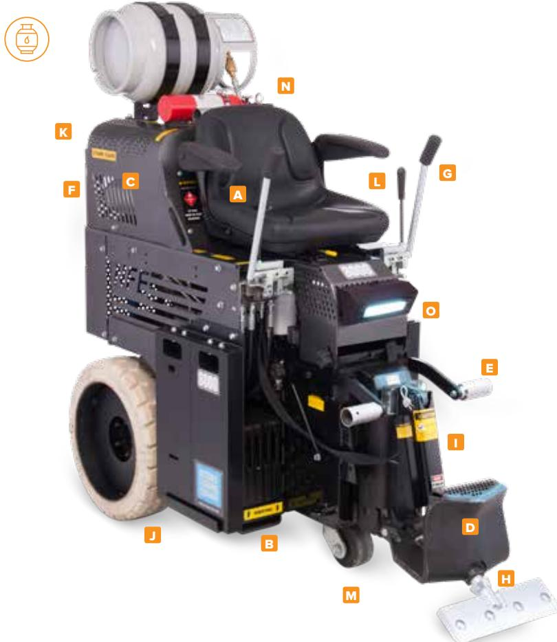
This 2,842-pound scraper rivals other manufacturers' heavier machines. Different from scrapers that are powered using a hydrostat drive system, the 8000 offers the speed and power of propane while also combining patented carbide angle-shank technology with the added efficiency of dual-lift hydraulic slide plates. Consistent torque sets the operational standard for high removal rates, and each machine undergoes a rigorous quality assurance program including emissions certification.
